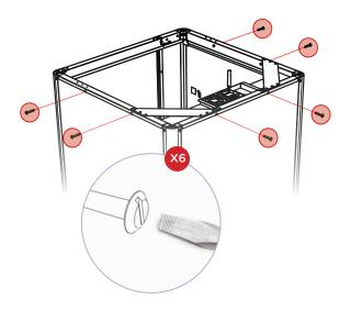
**6.** Once the roof frame is in place, use the flat head screwdriver to fully tighten all of the exterior M8 x 55 flange head bolts (16370). Bolts should be secure, but stop tightening if the wall panels begin to dimple.
