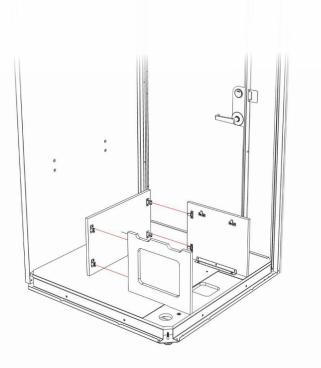
**4.** Tighten the (4) M8 x 35 button head cap screws (16840) on the seat frame right side and seat frame left side.
