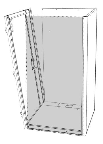
**10.** Use a flat head screwdriver to fasten the door to the left and right walls with (4) M8 x 55 flange head bolts (16370). Fasten the top left and right bolts first, then fasten the lower left and right bolts. Loosely tighten for now, you'll secure later.
