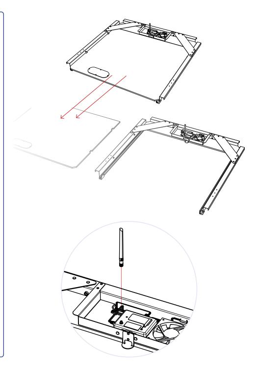
**3.** Orient the roof frame with the fan towards the back wall panel.
