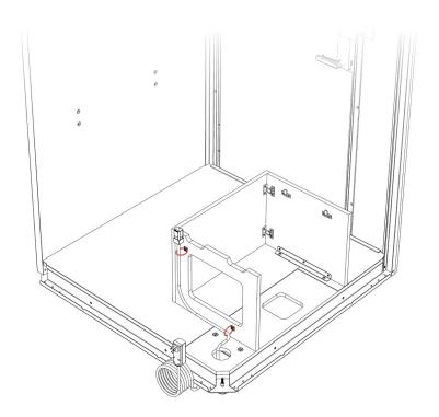
**6.** Place the seatback on its side. Use a Phillips head screwdriver and (2) 1/4" x 2" Phillips pan head screws to fasten the seatback to the seat base.
