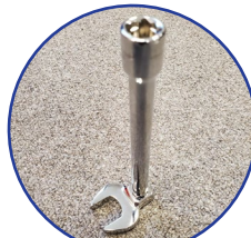
3/8" drive, 3/4" crowfoot wrench + wrench extension
