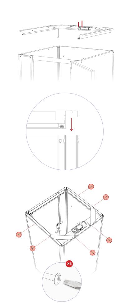
6. Once the roof frame is in place, use the flat head screwdriver to fully tighten all of the exterior M8 x 55 flange head bolts (16370).Bolts should be secure, but stop tightening if the wall panels begin to dimple.
