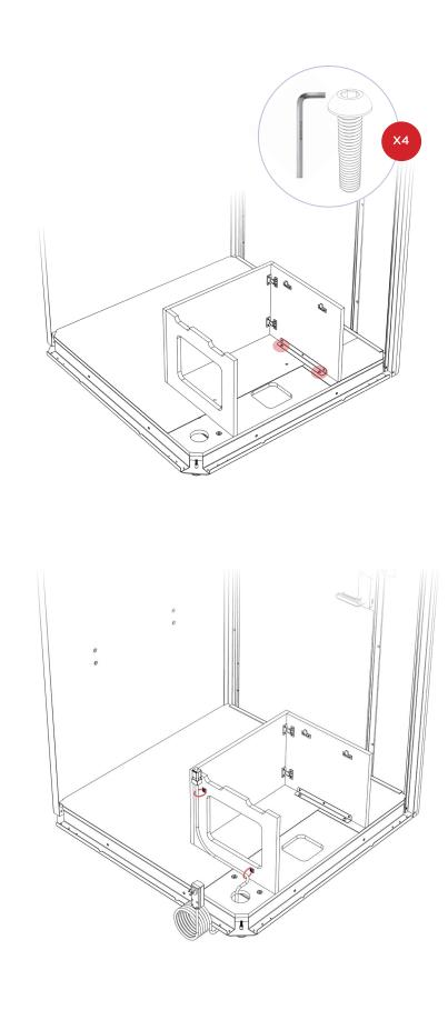
6. Place the seat back on its side. Use a Phillips head screwdriver and (2) 1/4" x 2" Phillips pan head screws to fasten the back to the seat base.
