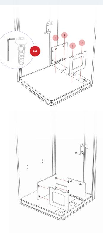
**4.** Tighten the (4) M8 x 35 button head cap screws (16840) on the seat frame right side and seat frame left side.
