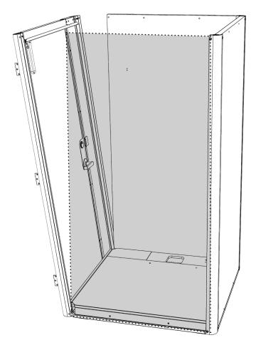
**10.** Use a flat head screwdriver to fasten the door to the left and right walls with (4) M8 x 55 flange head bolts (16370). Fasten the top left and right bolts first, then fasten the lower left and right bolts. Loosely tighten for now, you'll secure later.
