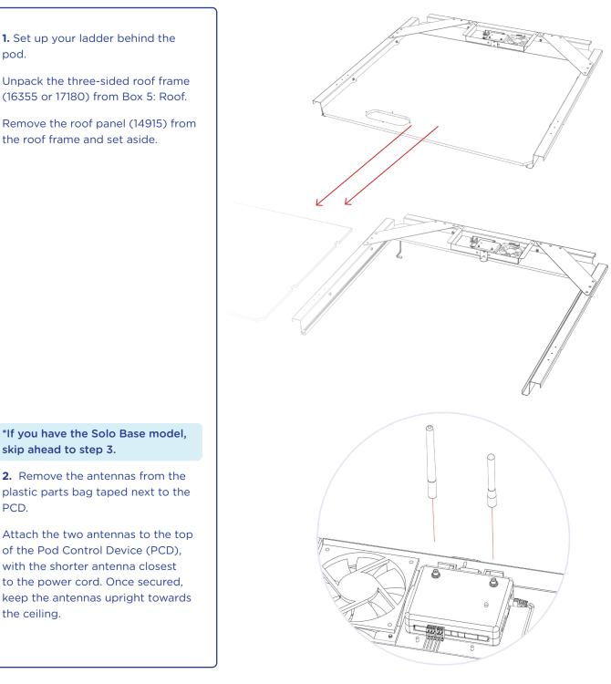
**3.** Orient the roof frame with the fan towards the back wall panel.
