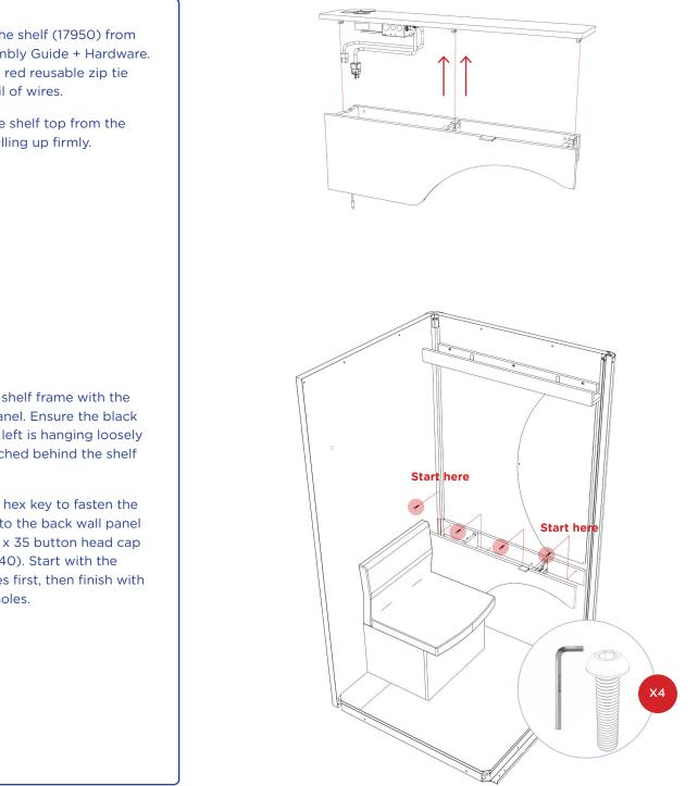
1. Remove the shelf (17950) from Box 1: Assembly Guide + Hardware. Remove the red reusable zip tie from the coil of wires.
