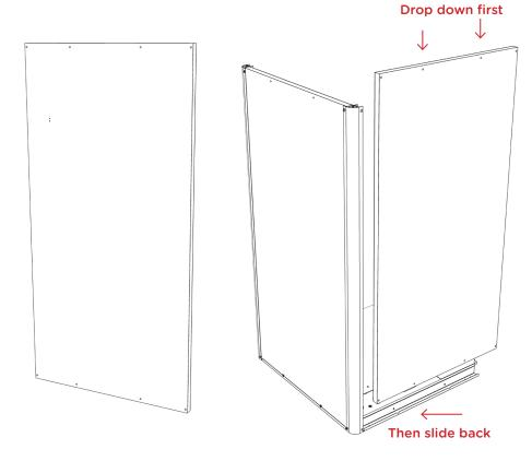
**4.** Use a flat head screwdriver to fasten the left wall panel to the foundation and back wall with (4) M8 x 55 flange head bolts (16370). Start from the top left to ensure the pod wall is stable. Loosely tighten for now, you'll secure later.
