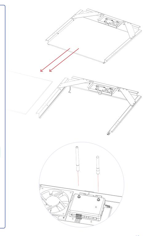
**3.** Orient the roof frame with the fan towards the back wall panel. The antennas should face the ceiling (not applicable to the Solo Base model).
