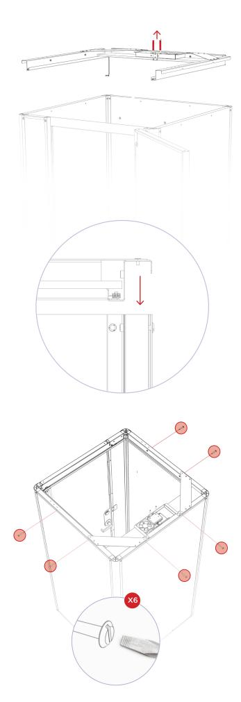
**6.** Once the roof frame is in place, use the flat head screwdriver to fully tighten all of the exterior M8 x 55 flange head bolts (16370). Bolts should be secure, but stop tightening if the wall panels begin to dimple.
